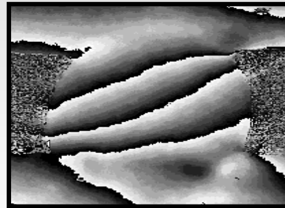
Local Displacement Field by Micro-Moire Interferometry
