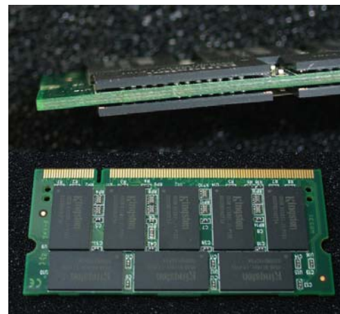
Figure 2 Memory module showing components mounted as Ball Grid Arrays (BGAs). (Photo provided by Helge Kristiansen, Conpart)
